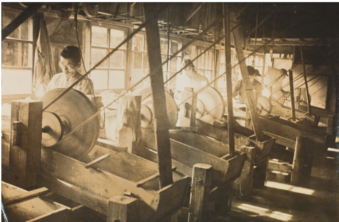
Fig.7 : Glass cutting workshop at Horiguchi Glass Inc., Tokyo, mid-twentieth century, with several lathes driven by one electric motor. The equipment and layout here is very similar to the original British cutting workshop design of the nineteenth century. Courtesy of Horiguchi Kiriko Inc.
